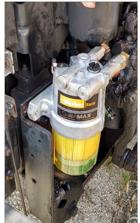
Fed Ex delivery truck retrofit. GreenMAX assembly part number used, 6600R10.
